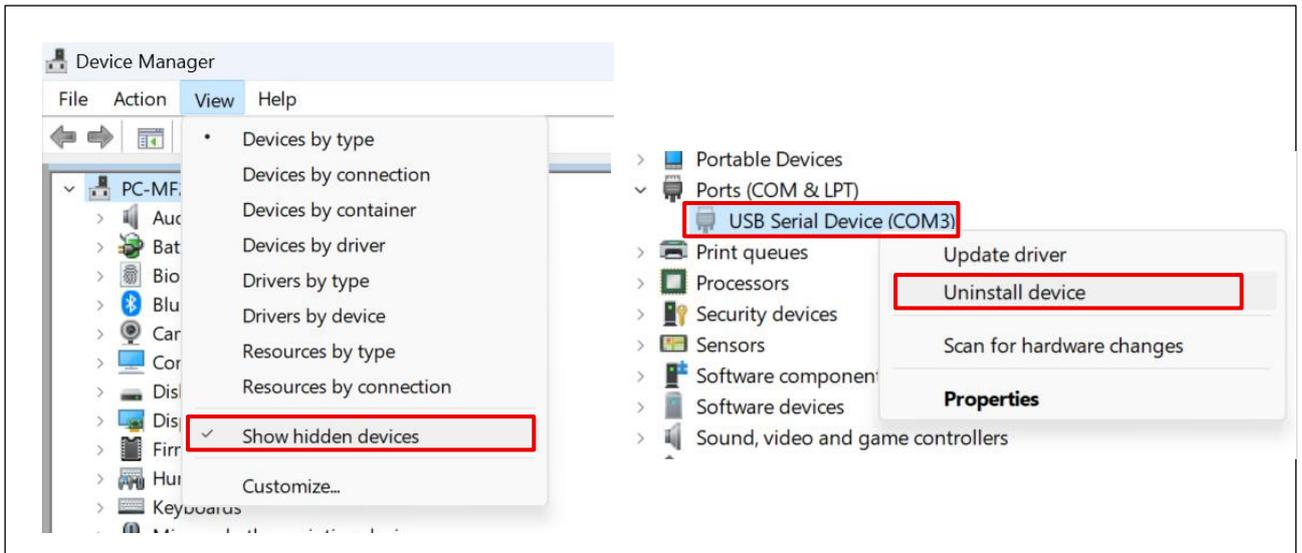
Figure 26: Device Manager – Show hidden devices / Uninstall device
